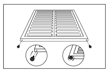
**STEP 1:** Do not remove protective film yet. Place front panel face down. Lay it on the flattened box to avoid scratching the screen. Screw the rubber mounts into the holes on either side of the bottom frame.
