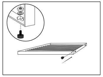
**STEP 5:** Lay the remaining side panel on the flattened cardboard.Install the rubber mount on the rear side of the side panel. Use a washer and nut.
