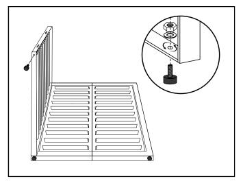
**STEP 3:** Install the rubber mount on the rear side of the side panel. Use a washer and nut.
