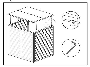
**STEP 7:** Align the hinged panel so the holes align with the holes on the rear side of the base. Secure using the hex head screws, nuts, and washers supplied. Use an Allen key to tighten the screws.
