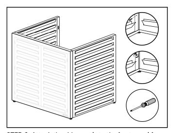
**STEP 6:** Attach the side panels to the front panel frame using the Phillips head screws.
