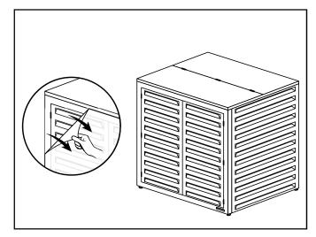
**STEP 8**: Remove the protective film from the front panel.
