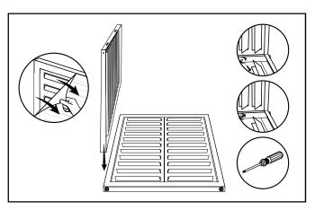
**STEP 2:** Remove the protective film from the side panels. Attach ONE side panel to the front frame using the Philips head screws. Ensure the louvres match the direction of the front panel.
