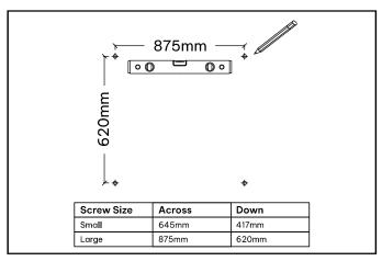
**STEP 2:** Mark the wall according to the size chart provided and install suitable wall anchors (not included). Screw the bolts in almost all the way, leaving a 3mm gap to fit the 2mm thickness of the aluminium.
