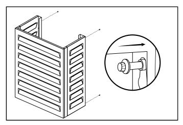
**STEP 3:** Once the wall anchors are securely installed, hang the screen by lifting it and slotting the wall bolts into the eyelet cutouts on the back of the screen. Tighten the wall bolts securely.
