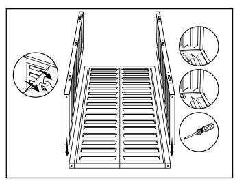
**STEP 2:** Remove the protective film from the side panels. Attach the side panels to the front frame using the Philips head screws. Ensure the louvres match the direction of the front panel.
