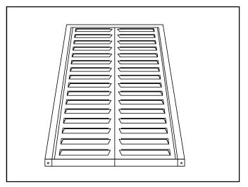
**STEP 1:** Do not remove protective film yet. Place front panel face down. Lay it on the flattened box to avoid scratching the screen.
