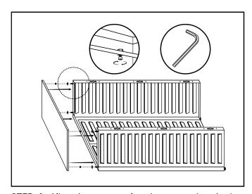
**STEP 4:** Align the top panel and secure using the hex head screws, nuts, and washers supplied. Use an Allen key to tighten the screws.
