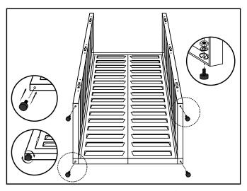
**STEP 3:** Install the rubber mounts. The 2 front mounts are screwed directly into the front door frame. For the rear rubber mounts, use the washers and nuts provided.
