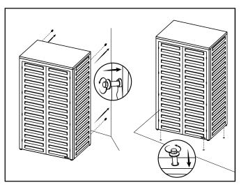
**STEP 6:** Mark the back wall and install suitable wall anchors (not included). If anchoring to the floor, use the holes on the bottom of the side panels.
